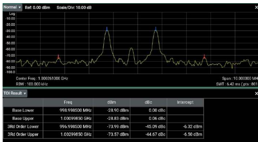
Figure 5.6 TOI Distortion Measurement Interface
