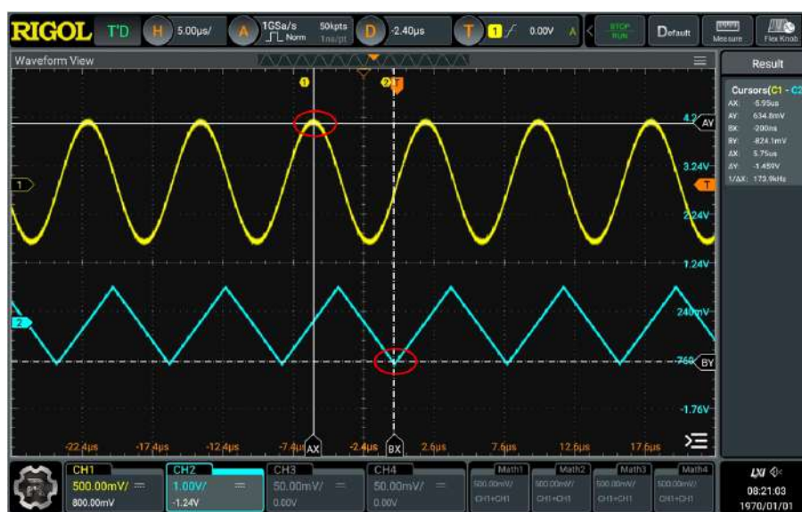
Figure 10.12 Track Measurement (before Horizontal Expansion)
