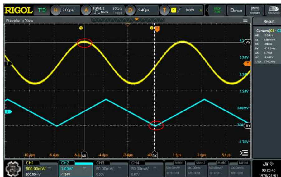
Figure 10.13 Track Measurement (after Horizontal Expansion)
