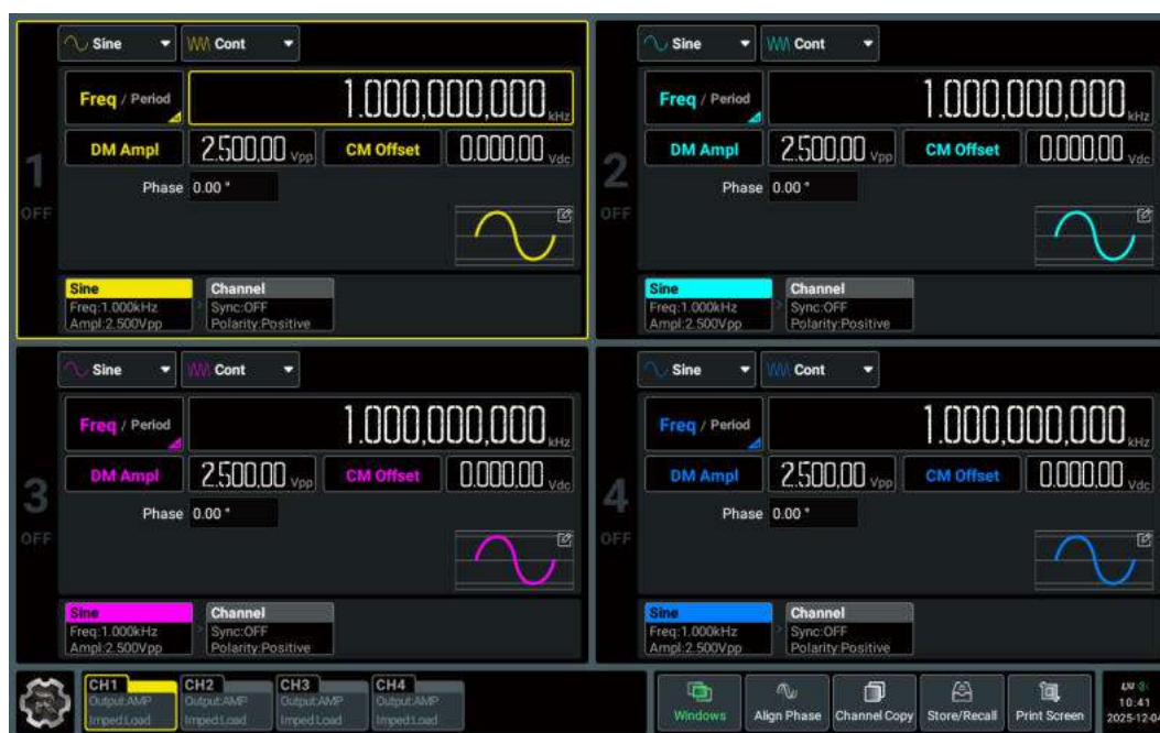
Figure 4.11 4-Channel Model User Interface - 4-Channel Display Mode
