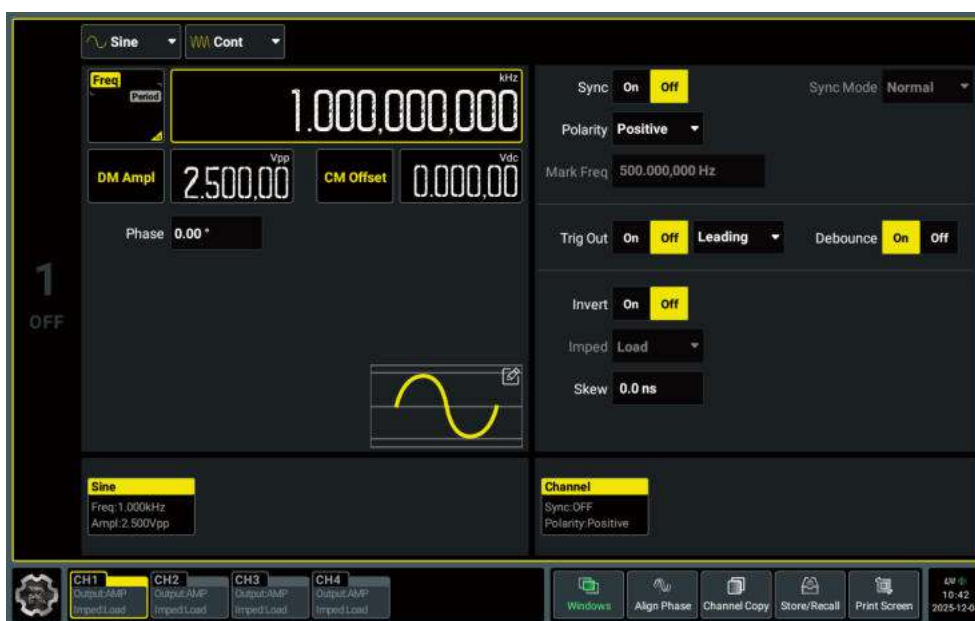
Figure 4.9 4-Channel Model User Interface - Single-Channel Display Mode
