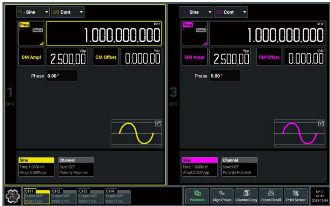
Figure 4.10 4-Channel Model User Interface - 2-Channel Display Mode
