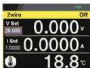
White: Temperature Control on with GTL-205A Connected
