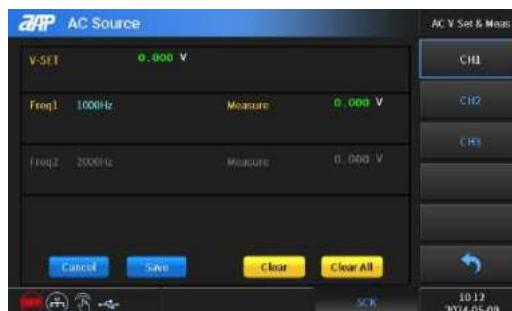
Select the calibrated gear to enter this interface. Select the corresponding channel. Only one channel can be calibrated at a time, and three channels cannot be calibrated simultaneously. Set the 420V file to 200V, input the corresponding voltage measurement value of each frequency in turn, and click Save,until 5KHZ. Repeat the calibration twice.
