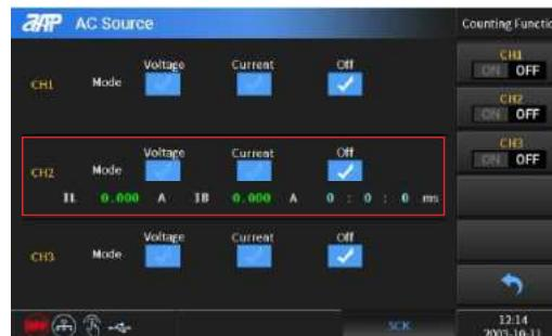
After the setting, press the [On/Off] key to turn on the output. The count starts from when output current has reached Ib setting and stop until the breaker or fuse is open, when the output current is less than IL setting.
