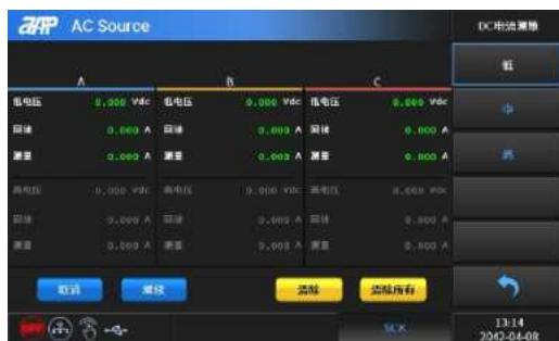
DC current measurement calibration point: low low current  $\pm 0.5A$ , high current  $\pm 0.8A$ ; Mid-range low current  $\pm 1A$ , high current  $\pm 5A$ ; High grade low current  $\pm 4A$ , high current  $\pm 16A$ .
