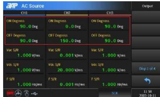
**ON Degress:** When the output is turned on, the ON degress of the output waveform can be set to 0~359.9°.
