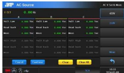
AC calibration point: 420V low voltage 50V, high voltage 300V; 210V Low voltage 50V, high voltage 150V. The calibration actual value and the readback value are the same calibration point.
