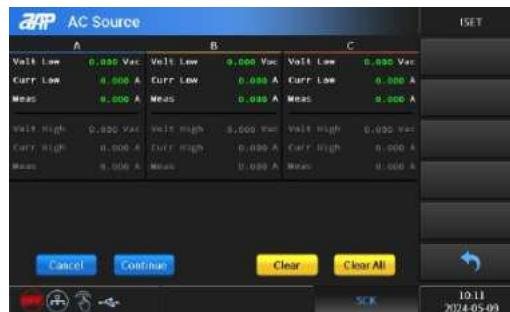
AC current setting calibration point: low current 4A, high current 16A.
