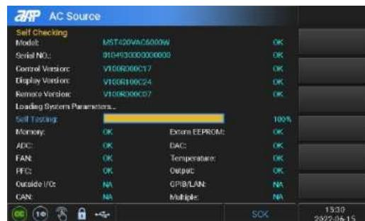
Please contact APM customer service for support if there are any failed items on this self-checking page. The diagnostics will take several seconds to complete. Once the unit completes the self-tests, the display screen will revert to the main page.
