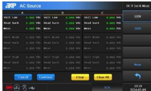
DC calibration point: 520V low voltage -400V, medium voltage 0V, high voltage 400V; 60V low voltage -200V, medium voltage 0V, high voltage 200V.
