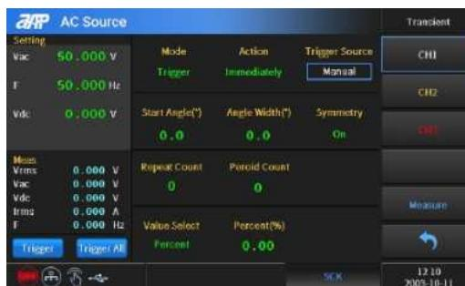
The Settings and measurements on the left side follow the Settings and measurements on the main interface.
