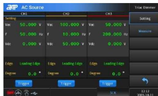
Set the Vac, F, Vdc, and I parameters on the main screen.
