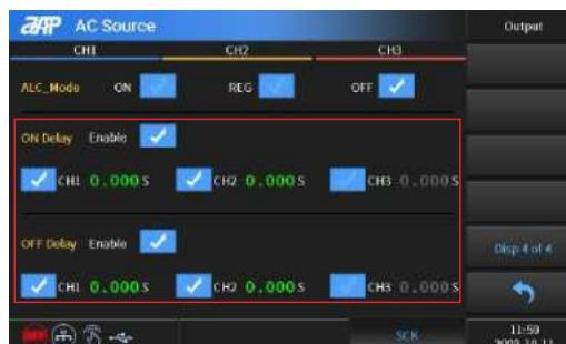
**ON Delay:** After this function is enabled, the Delay TAB is displayed on the main screen. You can control multiple channels to start output according to the set delay time.
