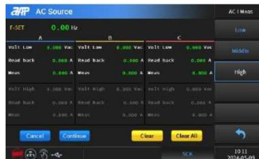
AC current measurement calibration point: low low current 0.5A, high current 0.8A; Mid-range low current 1A, high current 5A; High grade low current 4A, high current 16A. The frequency is set at 200Hz.
