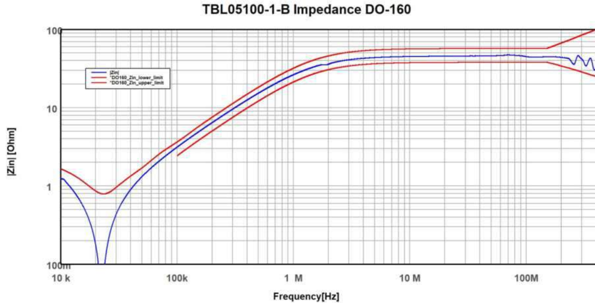
Picture 5: LISN impedance, 10 kHz – 400MHz; 50 \Omega // 5 \mu H; Jumper J1 open, Jumper J2 open, external 10 \mu F capacitor connected at the source port
