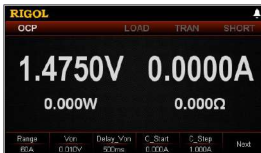
Figure 2-30 Main Interface of OCP Test Function
