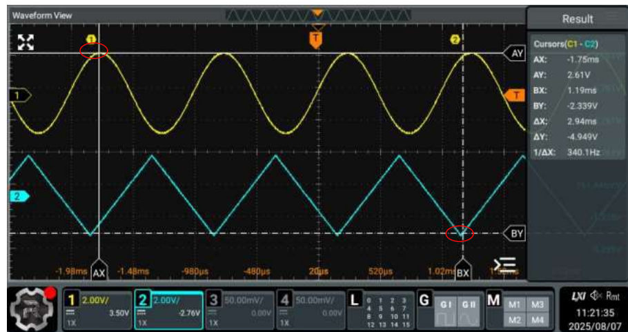
Figure 10.11 Track Measurement (after Horizontal Expansion)
