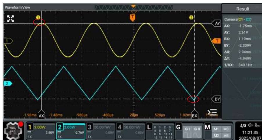
Figure 10.11 Track Measurement (after Horizontal Expansion)
