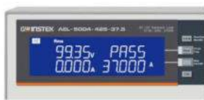
Turbo OFF, Short 100ms 37.5A Test result screen
