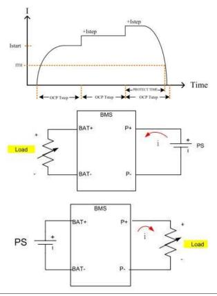
• Setting the BMS OCP ISTAR current, the upper 5 digit monitor display the "OCP", the middle 5 digit monitor display the "ISTAR", and lower monitor display setting value, the unit is "A". The range is 0.96A to the 600.00A, step 9.6mA by rotating the setting knob.
