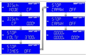
• Set the battery discharge CP mode, DISCH CP. The upper left LCD show "DISch", the lower left 5-digit display on the left displays "CP", the setting range is from 0.000W to full scale, resolution: 9.6mW.
