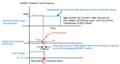
Figure C PEL-5006G-150-600 short-circuit current test procedure
