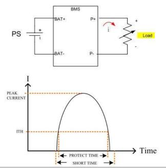
• Setting the BMS Short Time, the upper 5 digit monitor display the "SHORT", the middle 5 digit monitor display the "TIME", and lower monitor display setting value, the unit is "ms". The range is 0.05ms to the 10.000ms, step 0.01ms by rotating the setting knob.
