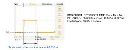
Figure D 4000mAh Power Bank Actual Short Circuit Test Waveform
