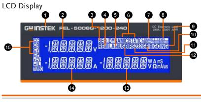
Model number and sink ranges The model number along with maximum voltage, current and power values are detailed in this position at the top of the load front panel.
