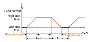
The dynamic waveform can also be set up via the optional computer interface. Dynamic waveform settings made from the front panel of the load module can also be saved in the memory of the PEL-5000G series Electronic Load. For the store/recall procedure and the computer command set please refer to the relevant operating manual for the PEL-5000G series Electronic Load.
