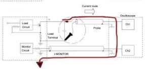
If the probes connection is reversed as shown above, a large current would flow through the probe and the internal circuitry of the oscilloscope is likely to be damaged.
