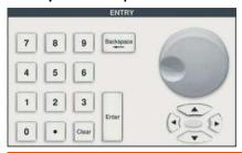
Rotary Knob and arrow Keys The rotary knob and arrow keys are used to increase or decrease the set values.
