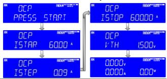
• ISTAR: Set the start current point, the LCD display shows "OCP" on left 5 digit LCD display, middle 5 digit LCD display "ISTAR", right 5 digit LCD display setting value, the unit is "A". The setting range is 0.00A to the full scale of the CC mode specification. The setting is by rotating the setting knob, resolution: 9.6mA.
