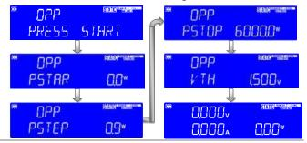
• PSTAR: Set the start power, the LCD display shows "OPP" on left 5 digit LCD display, middle 5 digit LCD display "PSTAR", right 5 digit LCD display setting value, the unit is "W". The setting range is 0.00W to the full scale of the CP mode specification. The setting is by rotating the setting knob, resolution: 96mW.
