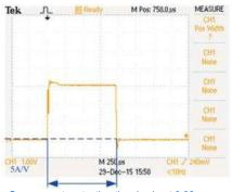
BMS OCP Pulse mode: SET OCP Istart = 15A, Tstep = 10ms, Istep = 0A, Ith = 1A PEL-5006G-150-600 test result: PEL-5006G-150-600 BMS: 0.981ms Oscilloscope: 0.980ms
