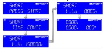
• Set the short test time, the LCD display show "SHORT" on left 5 digits LCD display, shows "TIME" on middle 5 digits LCD display, right 5 digit LCD display "CONTI", the unit is "ms".
