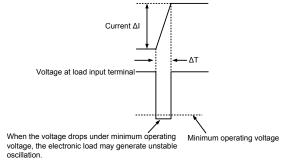
Waveform example: Generate unstable oscillation
