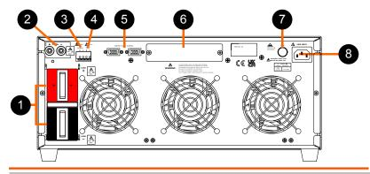
1 DC input terminal The positive (LOAD +) and negative (LOAD -) power input terminals are clearly marked. DO NOT confuse them with the smaller SENSE terminals.
