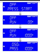
8. The UUT's output voltage drop-out lower than the threshold voltage (V-th setting), and the OPP trip point is between W\_Hi and W\_Lo limitation, then right 5 digits LCD display will shows "PASS", otherwise shows "FAIL".
