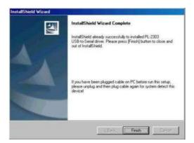
After the installation, connect the PEL-5000G series and PC with USB. Then select the item USB to Serial Port (COM3), set the BAUD-RATE and Flow control to 115200bps and Hardware to control PEL-5000G series with
