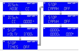
Set the battery discharge CC mode, DISCH CC. The upper left LCD shows "DISch", the lower left 5-digit display on the left displays "CC", the setting range is from 0.000A to full scale, resolution: 9.6mA.
