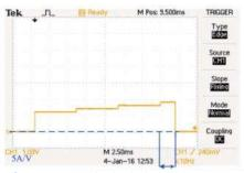
BMS OCP Pulse mode: BMS OCP: SET OCP Istart = 6A, Tstep = 5ms, Istep = 1A, Ith = 1A, Istep = 20A PEL-5006G-150-600 test result: 9A/2.013ms Oscilloscope: 2.015ms
