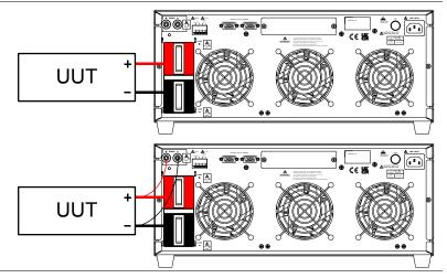
Typical connection of PEL-5000G series load module
