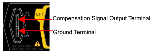
Figure 7.7 To Use the Compensation Signal
