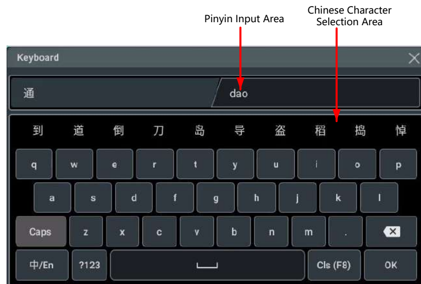
Figure 4.27 Chinese Input Interface
