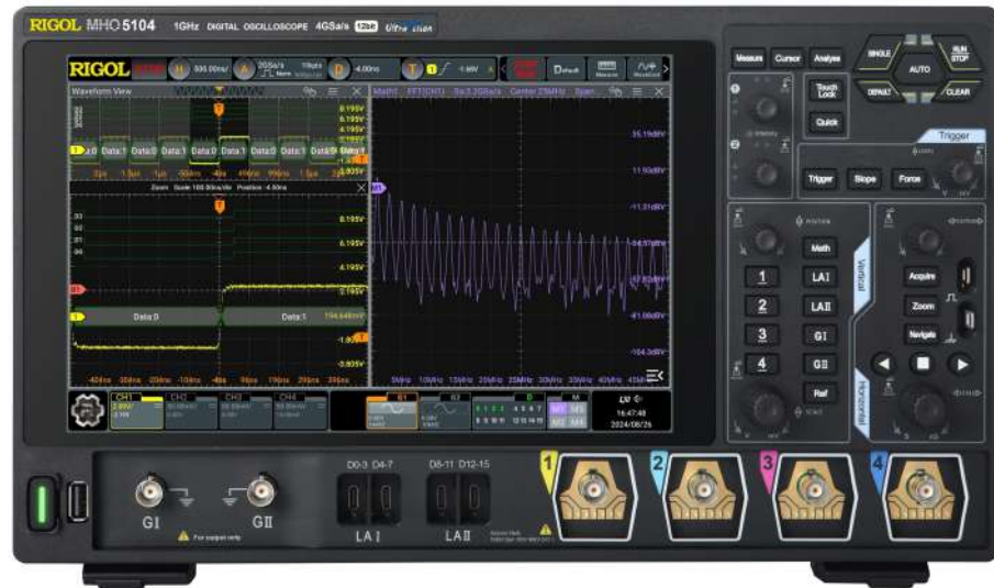
Figure 4.2 MHO5104 Front Panel
