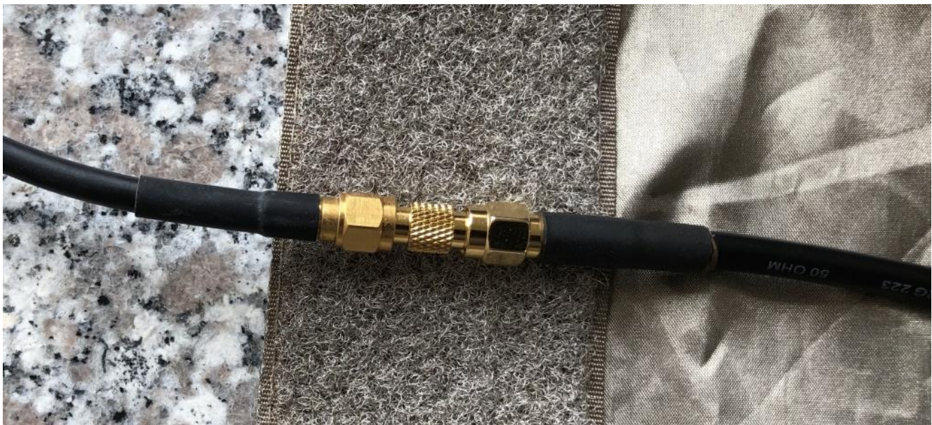
Picture 9: feed through using coaxial adapter
