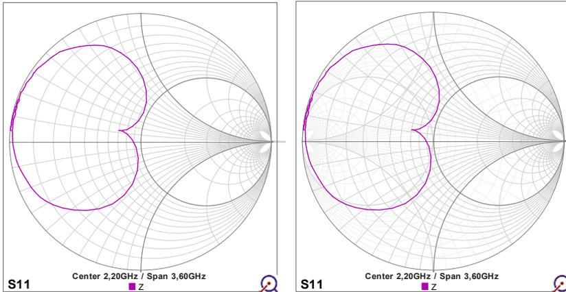
It is also possible to draw **admittance lines** that show what happens when impedances are connected in parallel. This is shown in the right graph above.
