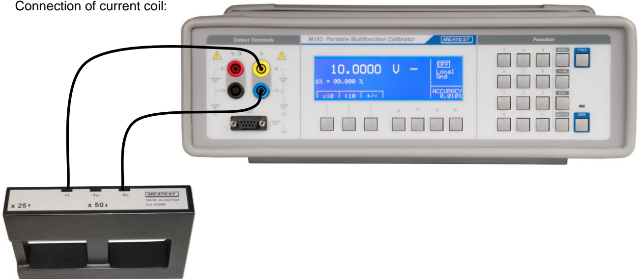
Fig. 25 Current coil connection
