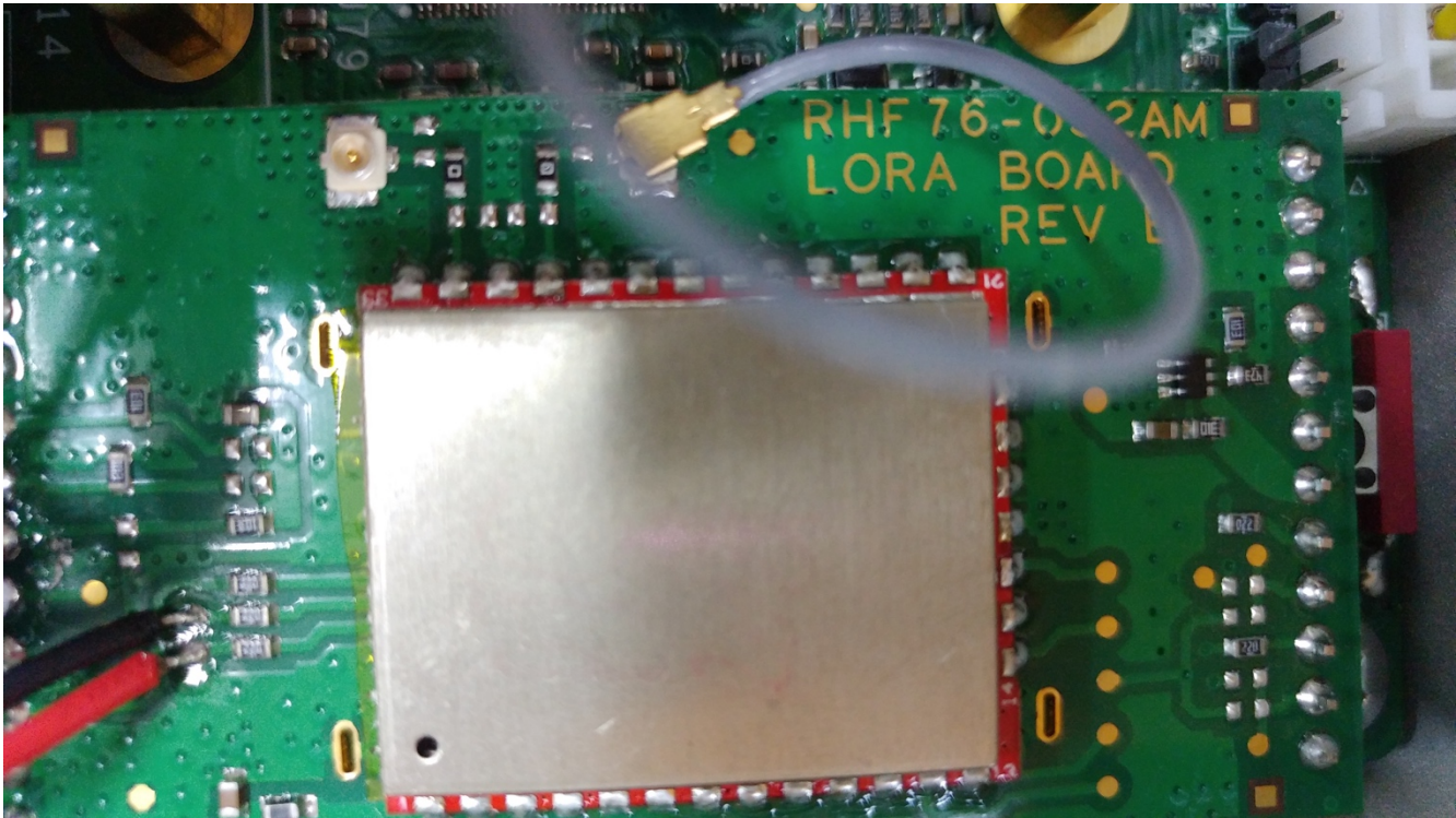
Antenna connected to LoRa modem high band connector
