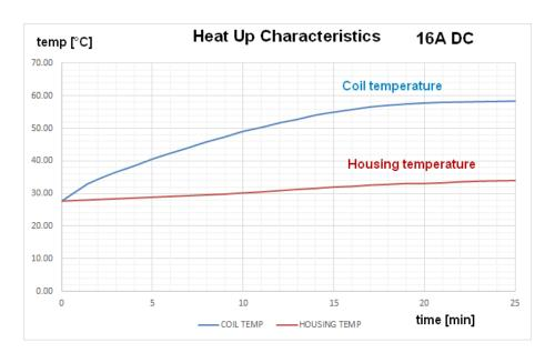
Picture 6: Coil and housing temperature at 16 A DC current
