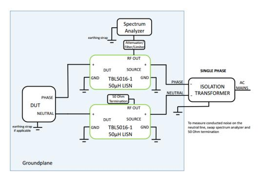
Picture 14: Measurement set up for single phase AC supplied equipment
