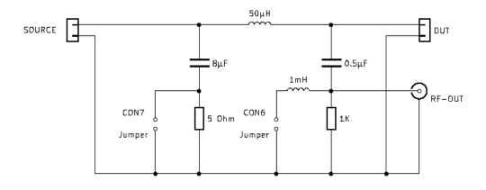
Picture 1: principle schematic
