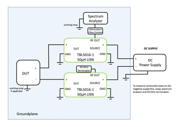
Picture 13: Measurement set up for DC supplied equipment
