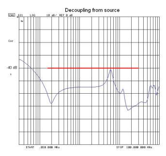
Picture 5: LISN Isolation, Source to RF out, 50Ω // 50μH
