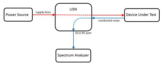
Picture 10: Basic diagram of a conducted emission measurement setup with a LISN
