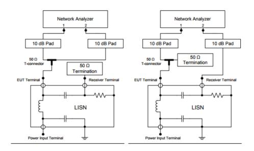
Reference measurement setup using network analyzer. Transmission measurement setup using network analyzer.
