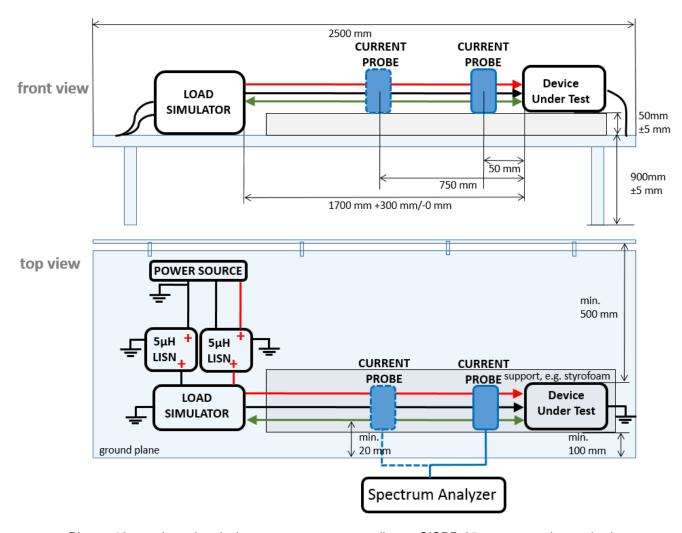
Picture 13: conducted emission measurement according to CISPR 25, current probe method
