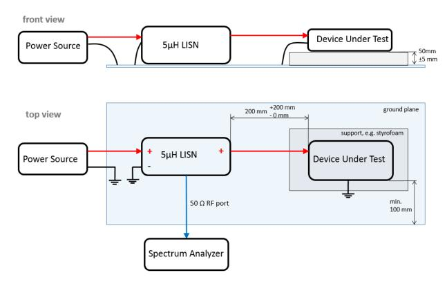
Picture 11: conducted emission measurement, voltage method, DUT with power return line locally grounded
