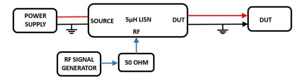
Picture 15: setup for RF injection
