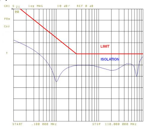
Picture 4: LISN Isolation, 100 kHz - 110MHz
