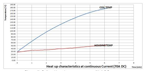
Picture 7: Coil and housing temperature at 70 A DC current
