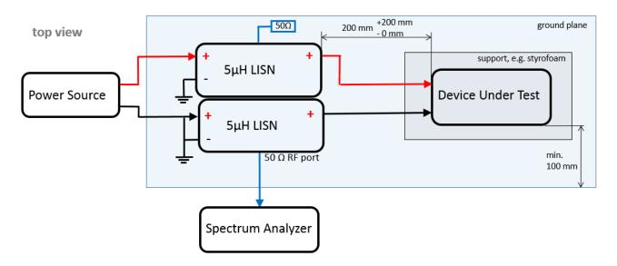
Picture 12: conducted emission measurement, voltage method, DUT with power return line remotely grounded
