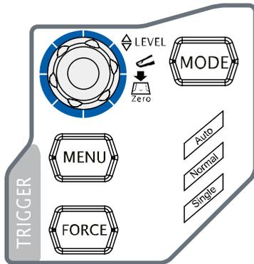
**MODE**: press this key to switch the trigger mode to **Auto**, **Normal** or **Single** and the corresponding state backlight of the current trigger mode would be illuminated.
