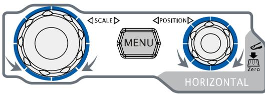
**MENU**: press this key to open the horizontal control menu under which to turn on or off the delayed sweep function, switch between different time base modes, switch between
