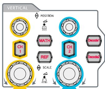
**CH1**, **CH2**: analog input channels. The 2 channels are marked by different colors which are also used to mark both the corresponding waveforms on the screen and the channel input connectors. Press any key to open the corresponding channel menu and press again to turn off the channel.
