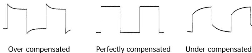
Figure 9 Probe Compensation
