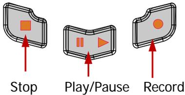
**Record:** press this key to start recording the waveform. At this moment, the red backlight of the key will start flashing. Besides, when the record constant on (Open) is enabled, the backlight will also keep flashing.
