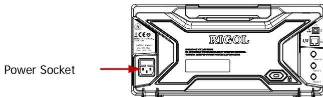
Figure 4 To Connect to AC Power Supply
