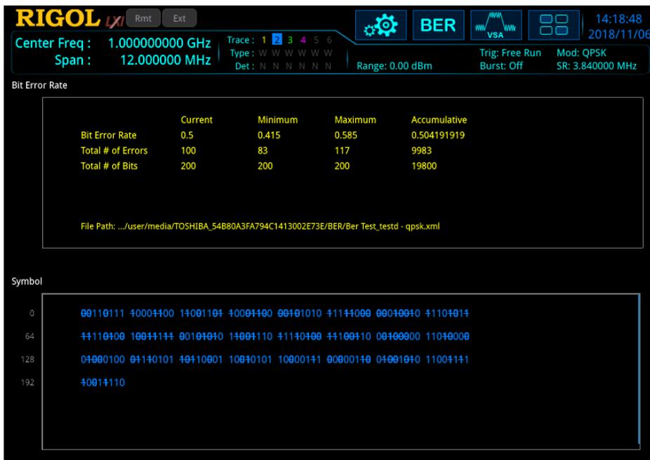
Figure 2-4 BER Measurement Results
